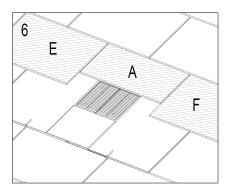
Alternatively, the ventilator position may be ideally located centrally over the gap between the 2 slates below the proposed ventilator position. Remove and cut the slates directly below the proposed position of the ventilator so that the slates do not protrude past the slate batten. Cut a 280mm wide gap in the batten as shown in detail 2.
